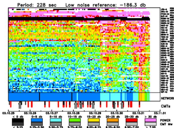
Signal power at 228 s period for stations of the Global Seismographic Network (GSN)
